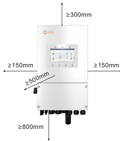
Figure 3.5 Inverter Mounting Clearances
